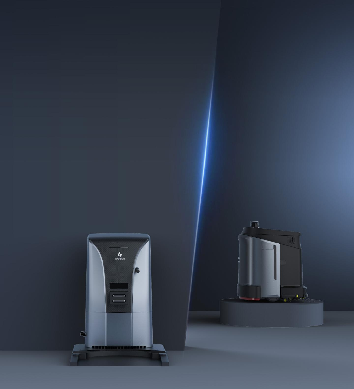
maximize uptime and minimize human intervention, the WS-03 allows the robot to automatically perform essential tasks such as power charging, water refilling, and discharge by simply docking with the workstation.
